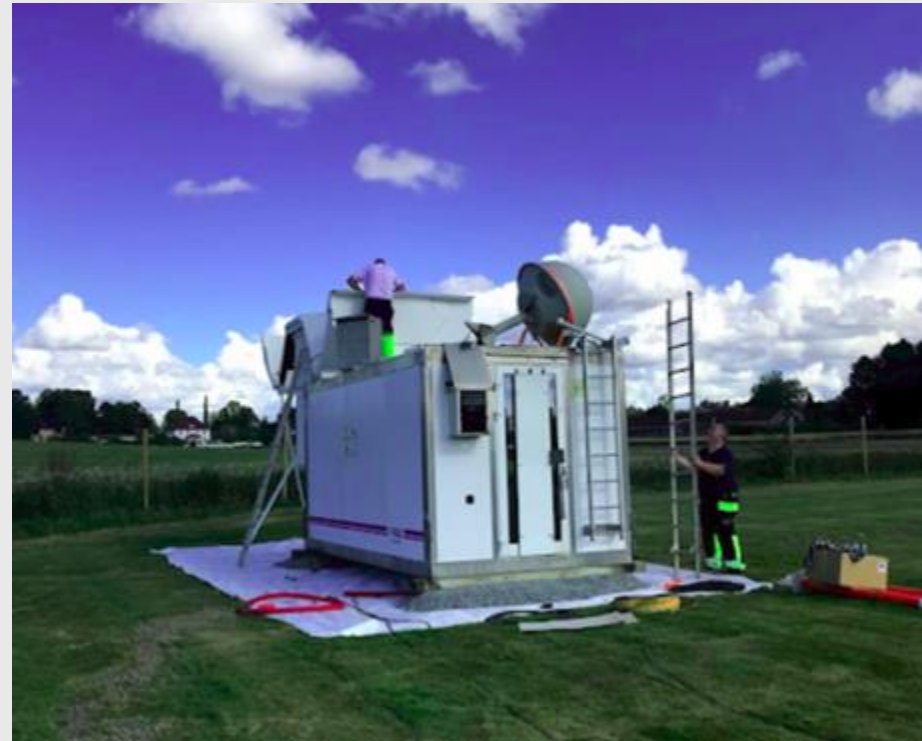
Figure 12: Deployment of radiosonde container Source: private
