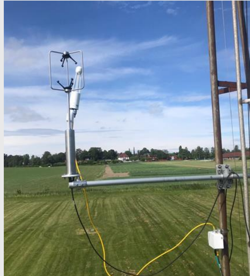
Fig. 8: Gill 3-D sonic anemometer and open-path LI-7500 gas analyser at 6 m height. Picture was taken during setup, the cables are fastened by now.
