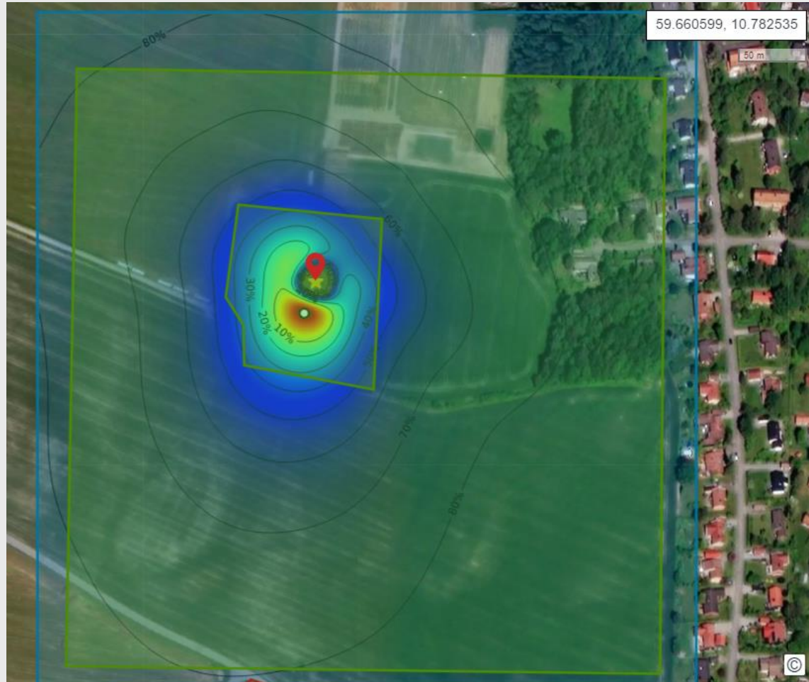
Fig. 16: Flux footprint for the summer season under unstable atmospheric stability.
