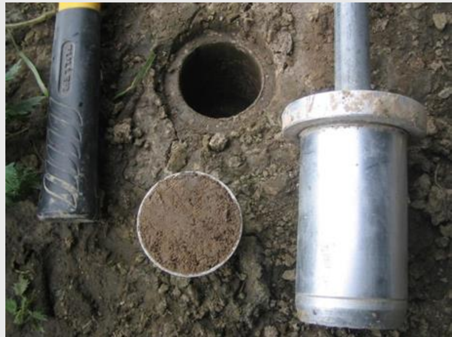
Figure 10: Bulk density core, stainless steel cylinder and hammer used for extracting soil cores Source: John Ballinger
